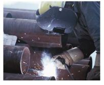
Metal gouging and lancing liberate particles of an unknown size and composition.
